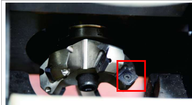
The square box contains the milling cutter blade.
